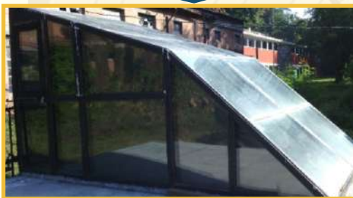
Head based storage Solar Kiln
